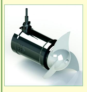
The GCWSM submersible mixer consists of a waterproof cast iron body with internal electric motor and a special impeller.
